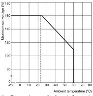
Note: The maximum coil voltage is the maximum voltage that can be applied to the relay coil.
